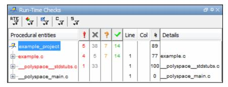
The file example.c is red because it has a run-time error. Polyspace software assigns each file the color of the most severe error found in that file. The first column of the table in the Procedural Entities View is the procedural entity (the file or function). The following table describes some of the other columns in the procedural entities view.
