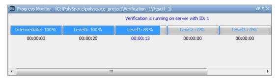
The progress monitor highlights the current phase in blue and displays the amount of time and completion percentage for that phase.
