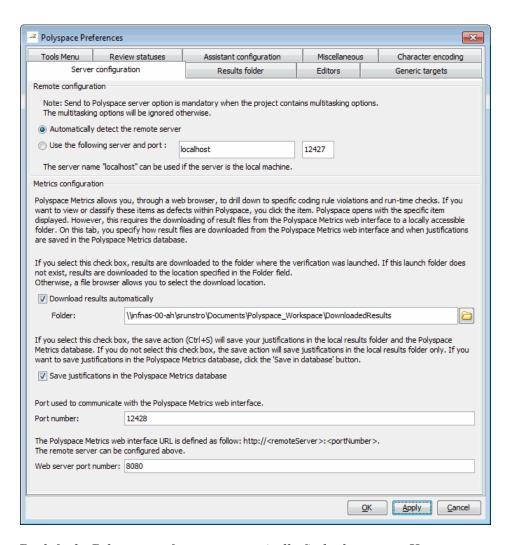
By default, Polyspace software automatically finds the server. You can specify the server by selecting Use the following server and port and providing the server name and port. For information about setting up a server, see the *Polyspace Installation Guide*.
