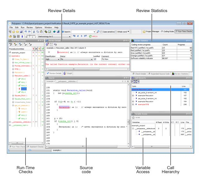
The Run-Time Checks perspective has six sections below the toolbar. Each section provides a different view of the results. The following table describes these views.
