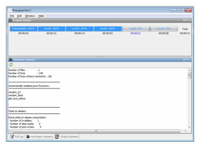
You can monitor the progress of the verification by watching the progress bar and viewing the logs at the bottom of the window. The progress monitor highlights the current phase in blue and displays the amount of time and completion percentage for that phase.
