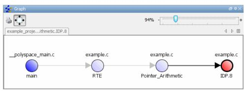
The code associated with IDP.9 is in Pointer\_Arithmetic. The generated main function calls RTE, which calls Pointer Arithmetic.
