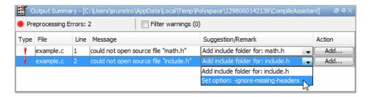
In this case, you can either add the missing include file, or set an option that will attempt to compile the code without the missing include file.
