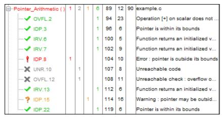
In the list of checks, each item has an acronym that identifies the type of check and a number. For example, in IDP.8, IDP stands for Illegal Dereferenced Pointer. For more information, see "Check Descriptions" in the *Polyspace Products for C Reference*.
