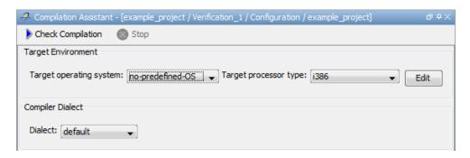
**2** In the **Target processor type** drop down menu, select i386.
